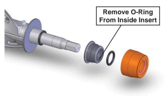
Figure 3-6 Rear Seal Removal
