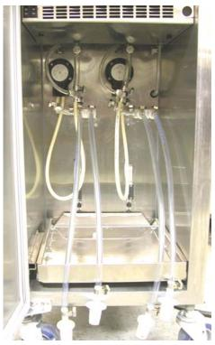
Figure 2-7 Completed BCS Hose Assembly
