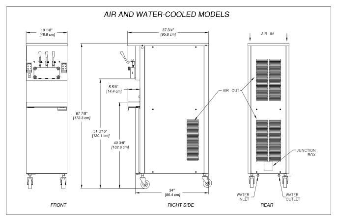
Figure 1-2 Machine Specifications
