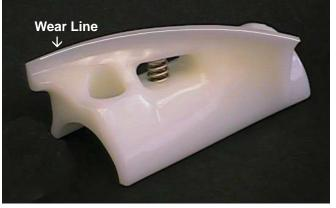
Figure 3-3 Auger Flight Wear
