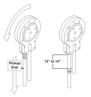
Figure 4-3 Pump Hose Reposition
