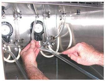
Figure 3-18 Cleaning Air Tube
