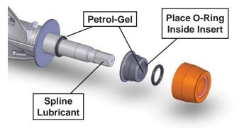
Figure 3-7 Rear Seal Lubrication
