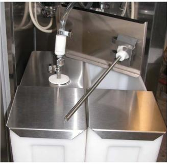
3. Connect elbow fitting to free end of tubing. Connect opposite end of elbow to 1/4" ID tan tubing on the left side of pump head. Secure with hose clamps (see Figure 2-3 and 2-4).
