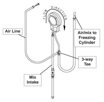
Figure 3-15 Mix Pump Hose Routing
