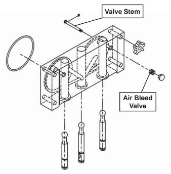
Figure 3-4 Front Door Disassembly
