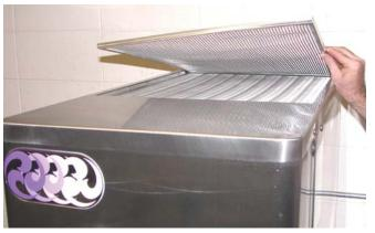
Figure 4-4 Removing Condenser Filter
