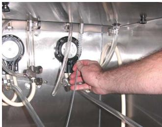
Figure 3-19 Cleaning Feed Tube
