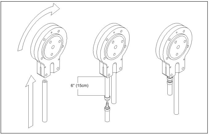
Figure 2-3 Mix Hose Installation
